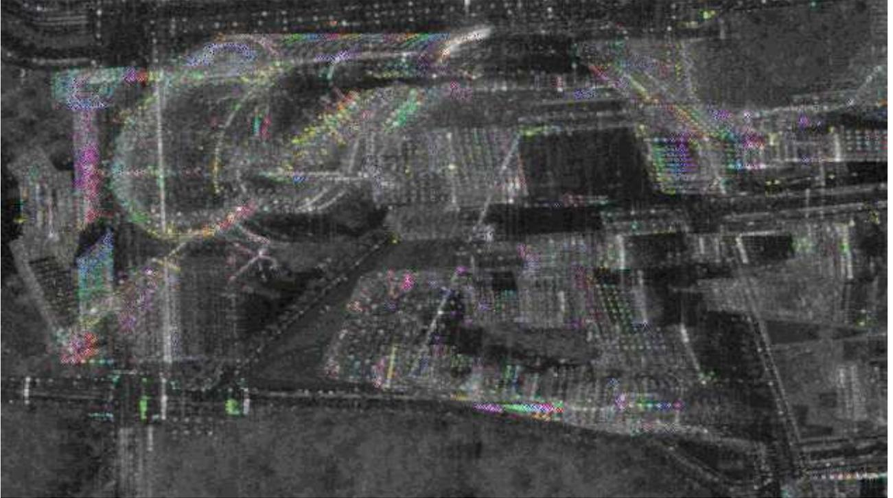
Figure 1. Phase of one interferogram of the stack overlaid on the mean amplitude image.
