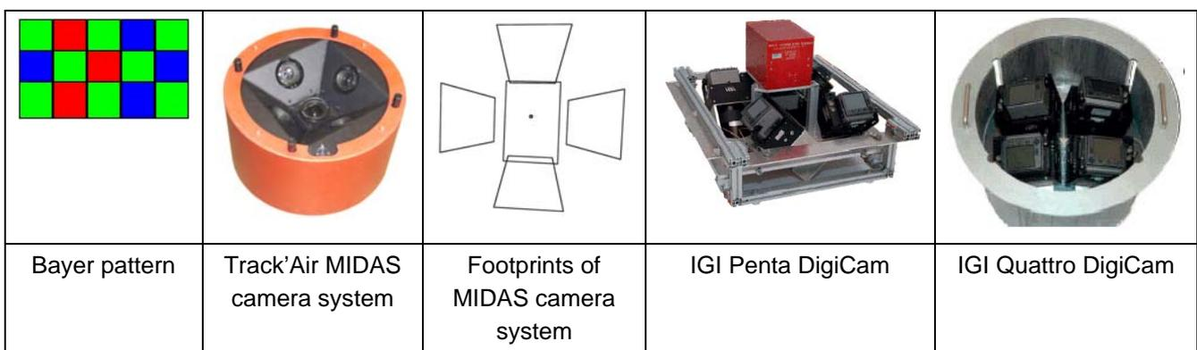
**Fig. 2.** details of mid-format cameras and camera systems
