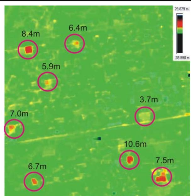
**Fig. 5.** filtered DSM height difference GeoEye from 2009-09-15 – IKONOS from 2008-05-24
