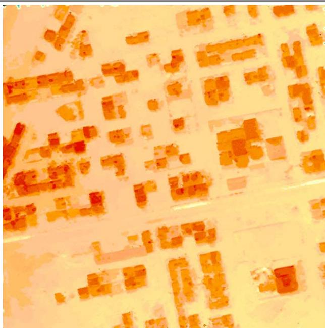
**Fig. 4.** color coded urban DSM generated by semi global matching with GeoEye-1 stereo pair
