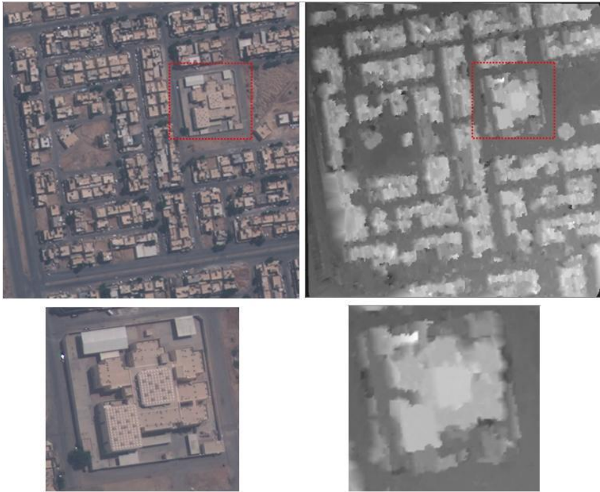
Fig.3: Left hand side: GeoEye-1 image, grey value coded DSM generated by LSM algorithm on right hand side; lighter gray levels correspond to higher elevations
