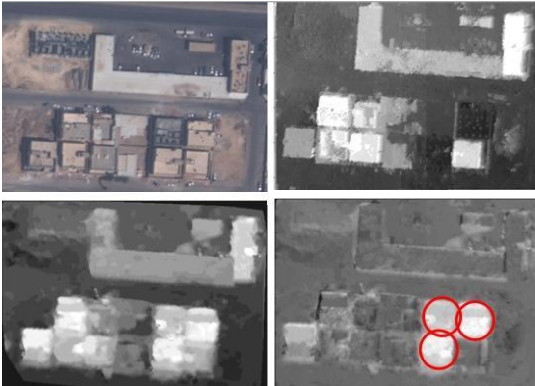
Fig. 6: Upper left: part of GeoEye-1 image, Upper right: grey value coded reference DSM, lower left: grey value coded GeoEye-1 DSM, Lower right: grey value coded DSM differences
