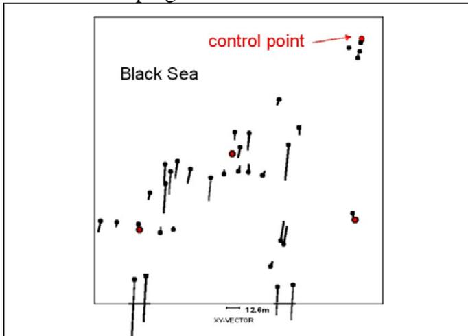
Fig. 6: 3D-affine transformation with 4 GCP describing nearly a tilted plane
