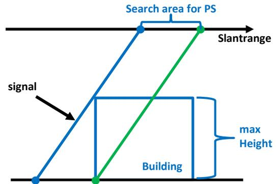
Figure 5. Geometric configuration for the pre-selection of PS based on a simple building model
