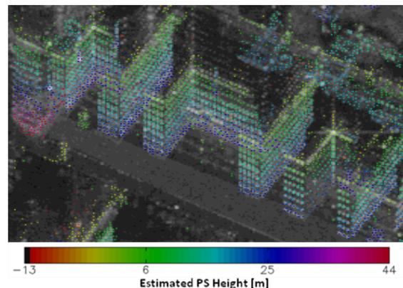
Figure 2. Mean amplitude image of the building under investigation overlaid with the PS identified for Grouping
