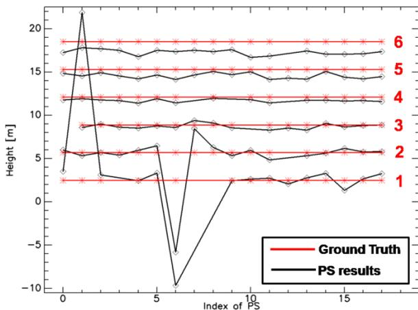
Figure 4. Height profiles for the lines located at Facade 2
