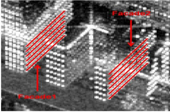
Figure 3. Manually selected profiles overlaid to the SAR amplitude image
