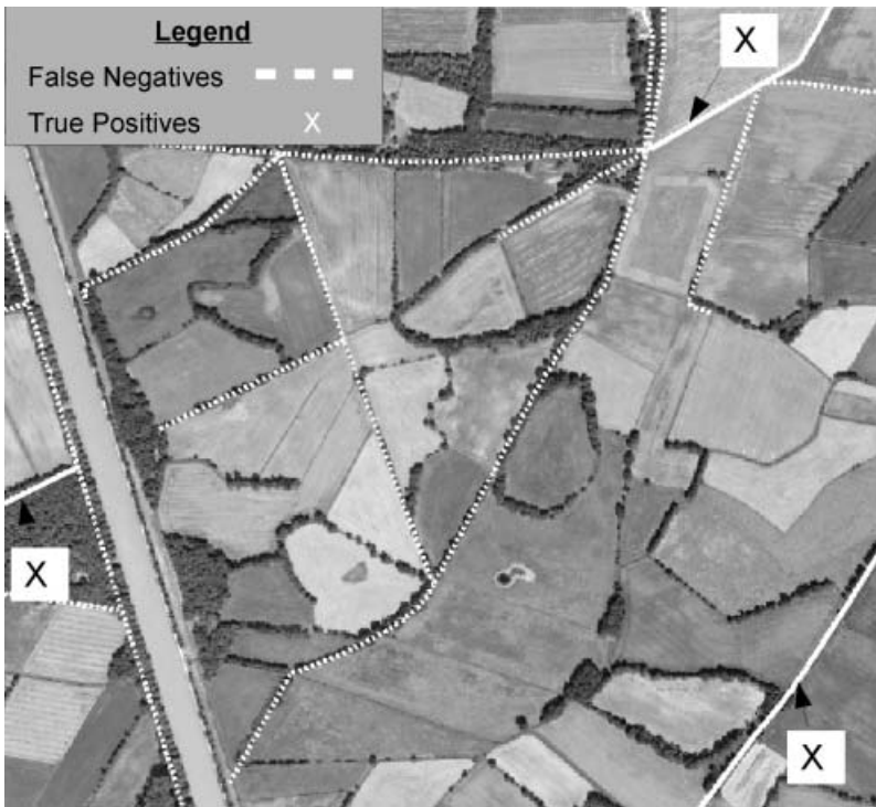
Figure 11. Limits of approach. False negative decisions for dead end roads, occluded by rows of trees.
