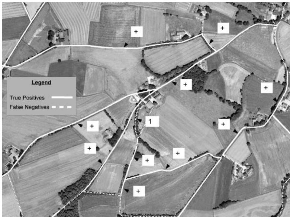
Figure 10. Example for true positives because of incorporation of rows of trees. The '+' mark objects which are additionally accepted after the rows of trees were incorporated.
