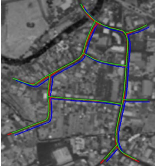
Figure 5. Image energy from a combination of intensity and height values (green: ground truth; blue: initialisation; red: final position)
