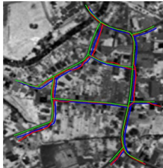
Figure 3. Image energy from intensity values (green: ground truth; blue: initialisation; red: final position)
