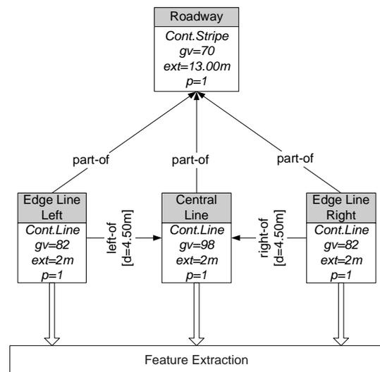
Figure 7. Adapted Object Model for Dual Carriageway 1.00m/pel
