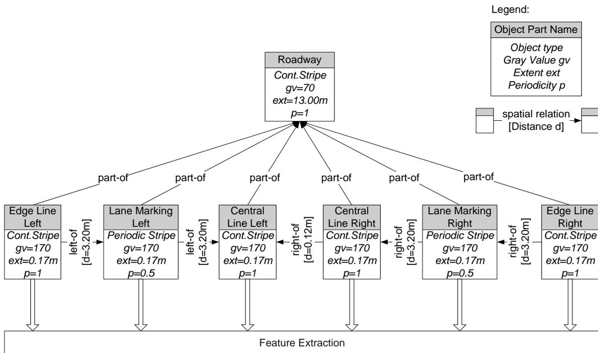
Figure 4. Original Object Model for Dual Carriageway in 0.03m/pel
