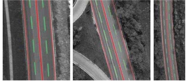
Figure 8. Extraction Results in 0.033m/pel – Reference (red: edge lines, green: lane markings)
