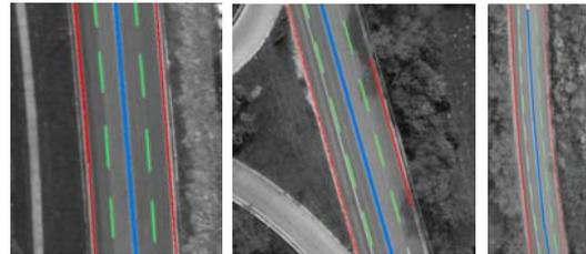
Figure 9. Extraction Results for 0.10m/pel (blue: central line, red: edge lines, green: lane markings)
