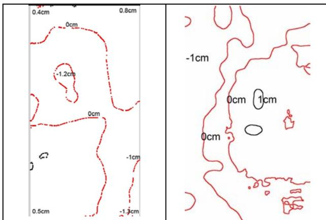
Figure 8: model deformation of DMCII-250, 5.4cm GSD, based on additional parameters 1-12 + 81-88
