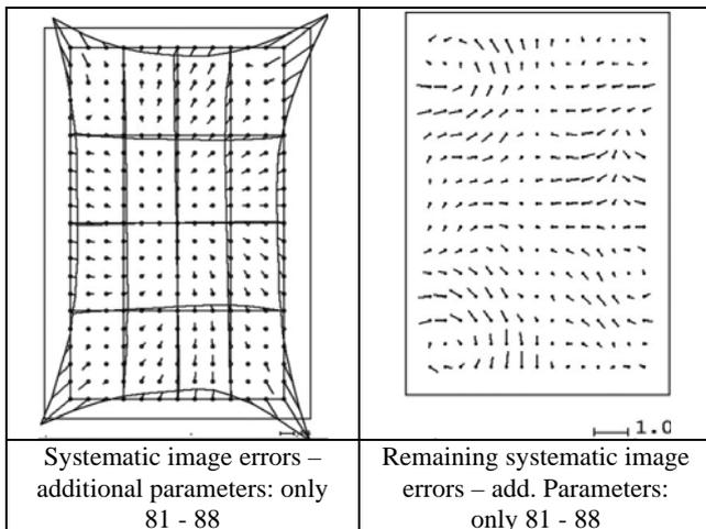
Figure 5: systematic and remaining systematic image errors UltraCam Eagle only with additional parameters 81 - 88
