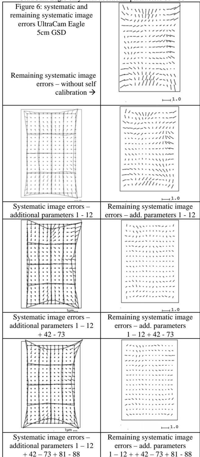
The UltraCam Eagle is fusing the 9 panchromatic sub-images of the 4 sub-cameras together. With the so called “monolithic stitching” (Ladstädter et al. 2010) the panchromatic sub-images are fitted to the green image which is based on one CCD-array with approximately linear three times lower resolution. This stitching improved the image geometry clearly against the former merging of sub-images; nevertheless the special additional parameters for the sub-images (parameters 32-73) have to be checked.
