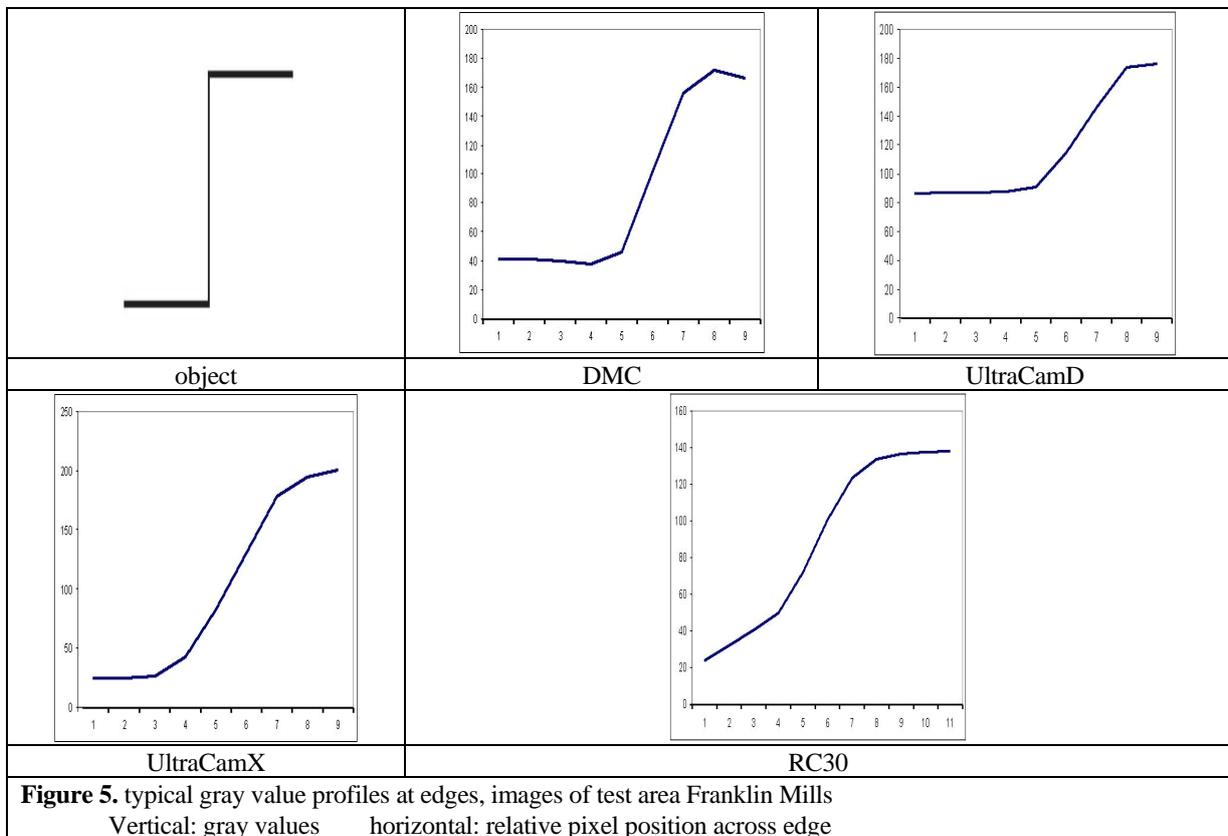
For the analysis an edge is specified by 2 points in the image (figure 4, center). All gray value profiles between these both points, perpendicular to the edge are used for the analysis. All gray value profiles of an edge are averaged before computation of the point spread function, reducing the noise especially of scanned photos.
