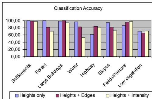
Figure 3: Accuracy of classification/segmentation
