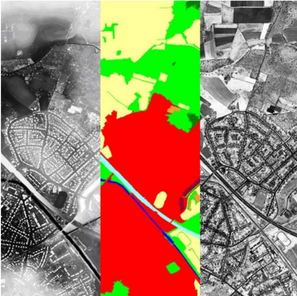
Figure 2: Segmentation result for variant (3) (left gray coded height, middle segmentation result, right intensity image of laser scanner data)
