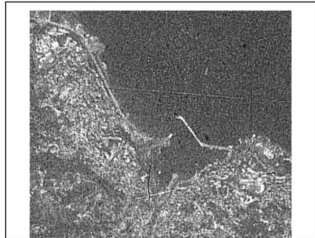
Fig. 9: sub-area of TK-350 digital image showing scratches and film grain
