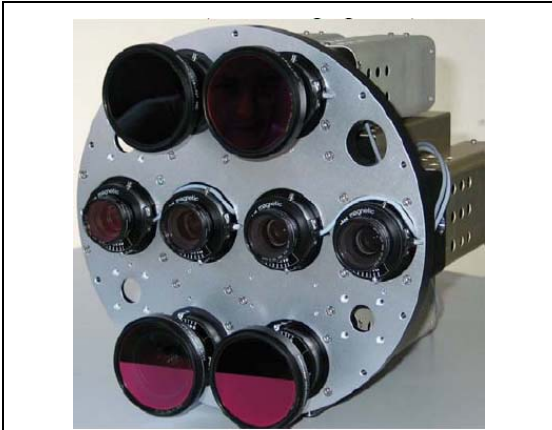
Fig. 7: configuration of UltraCam D lenses
