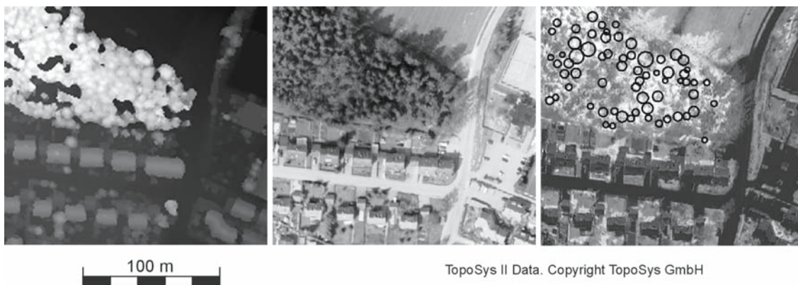
Fig. 17 Ravensburg data set. Left DSM. Middle Intensity channel of the colour-infrared image. Right Extraction results
