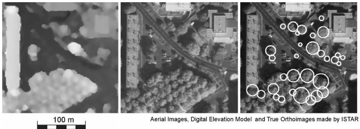
Fig. 16 Paris data set. Left DSM. Middle Intensity channel of the colour-infrared image. Right Extraction results
