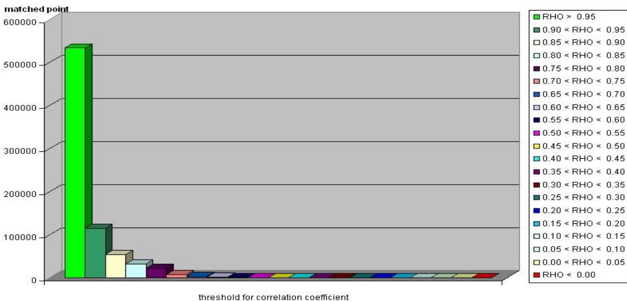
Figure5: Frequency distribution of correlation coefficients of least squares matching in complex areas with small and large building and trees, sub-matrix for least squares matching 10x10 pixels; step width = 3 pixels
