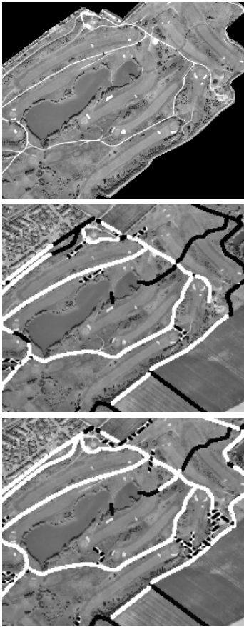
Fig. 4. Extraction results of the region SmallStructures : Original orthoimage (top) and evaluation with reference data with unsuitable (center) and suitable parameter set (bottom); White lines correspond to correctly extracted roads, black lines to non-extracted roads, dashed lines to incorrectly extracted roads.
