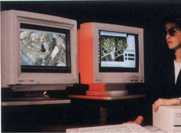
Figure 2: LH System Digital Photogrammetric Workstation (Copyright LH Systems)
