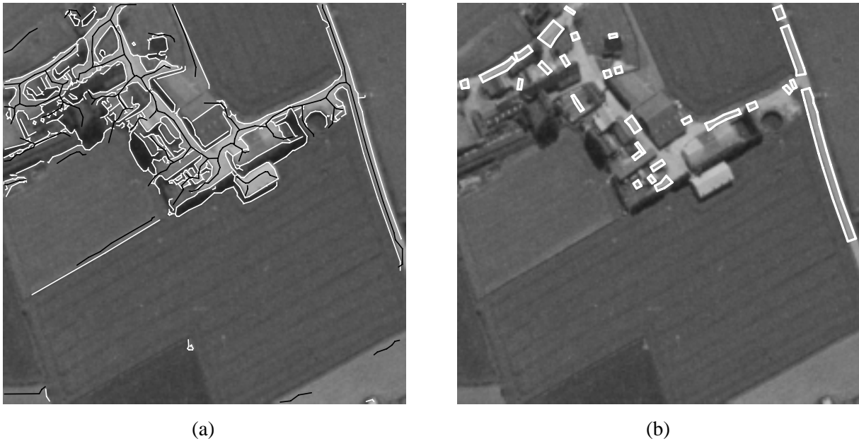
Figure 5: a) Input to the fusion: lines from coarse scale (black), edges from fine scale (white). b) Hypotheses for road segments.
