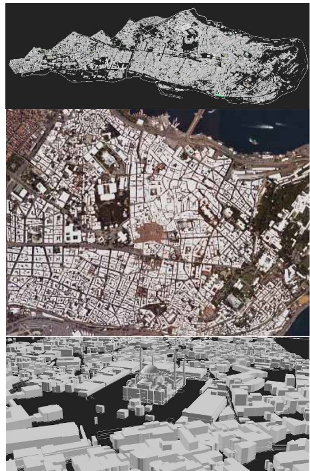
Figure 8. Combination of data from two different sources: 3D polylines of roofs based on aerial images and 3D polylines of facades from terrestrial laser scanning data
