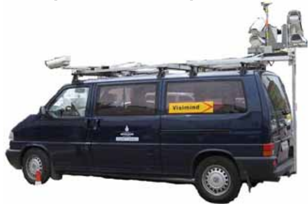
Figure 3. Sensor configuration on the mobile mapping van of VISIMIND AB
