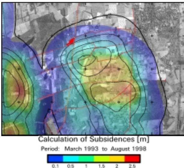
**Fig. 1:** HRSC-A ortho image (August 1998) and “*Calculation of Subsidence 1993–1998*”; overlay: red: GPS-points 1999, yellow: line levelling points, black: 1m-contour lines “*Calculation of Expected Subsidence 1993-2004*”.
