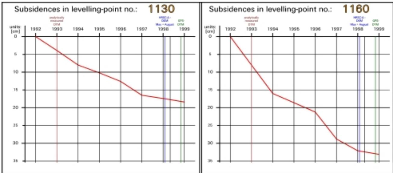
Fig. 7: Subsidence in levelling points no. 1130 and no. 1160 in the period from 1992 to 1999.
