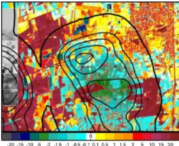
**Fig. 3:** Superimposition of Height Differences [m] (Analytical DTM 93 minus HRSC-A DEM 98) and HRSC-A data (left side); with an overlay of "Calculation of Expected Subsidence 1993-2004".
