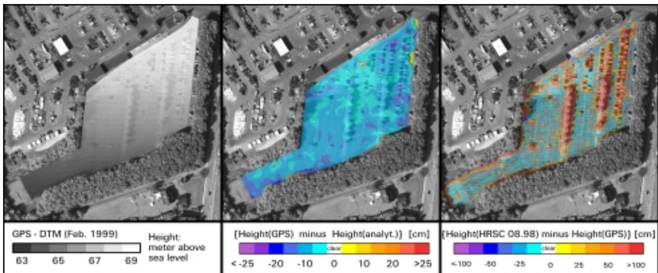
**Fig. 6:** DEM based on GPS-measurements 1999 (left), calculated differences between GPS measurements and analytical measurements 1993 (middle), calculated differences between HRSC-DEM and GPS measurements.
