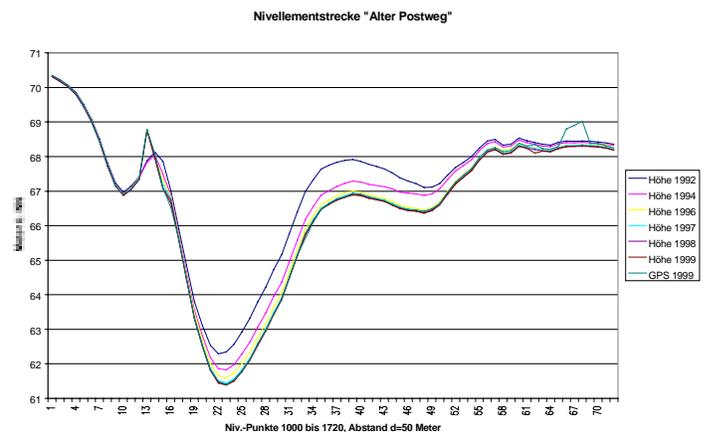
**Fig. 2:** Line levelling heights from 1992 to 1999 and GPS-heights 1999.
