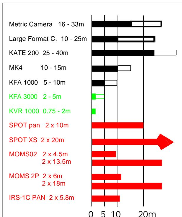
figure 1: ground resolution [m/lp] or size of 2 pixel
