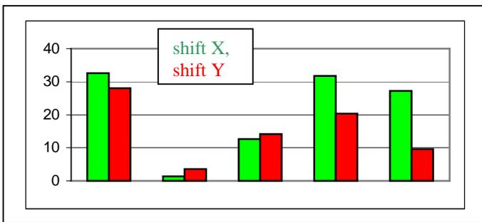
Figure 8: shift of the orthoimages after height correction against control points – Z-reference = mean height of control points (areas: Switzerland, USA, Malaysia, 2x Turkey)
