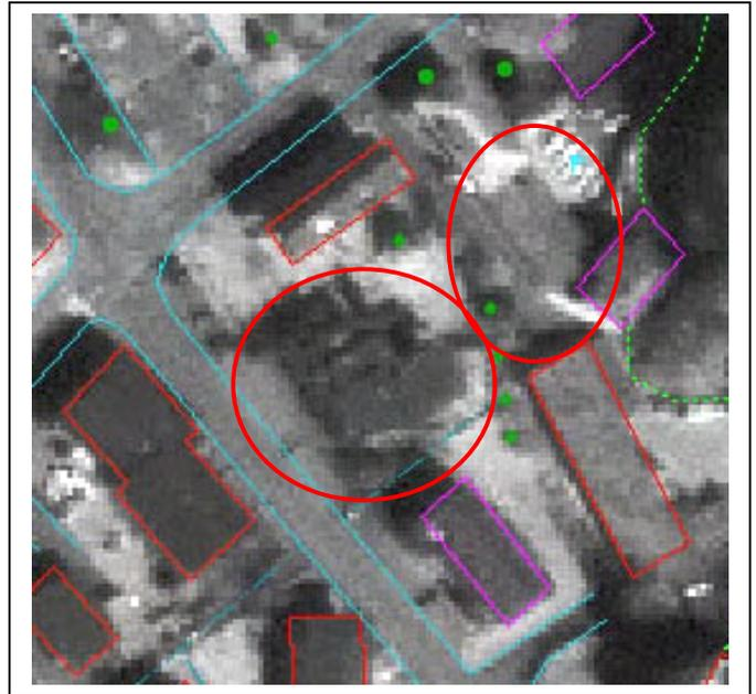
Figure 16: details of the line mapping with IKONOS image, encircled building not recognised
