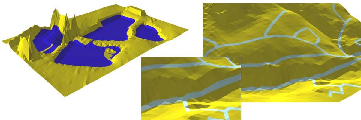
Figure 1: The integration of a DTM and 2D topographic vector data without considering the semantics of the objects; left: lakes, right: road network, exaggerated terrain
