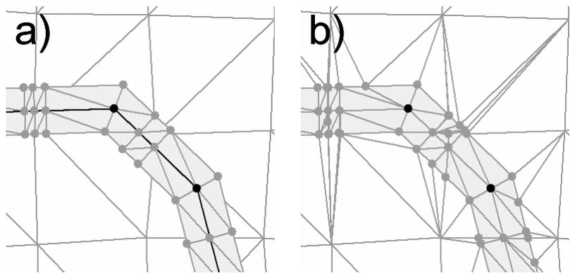
Figure 3: Integration of a DTM and a topographic object "road", a) original DTM TIN and object "road", b) intersection between DTM TIN and object, c) buffered object, d) integrated data set
