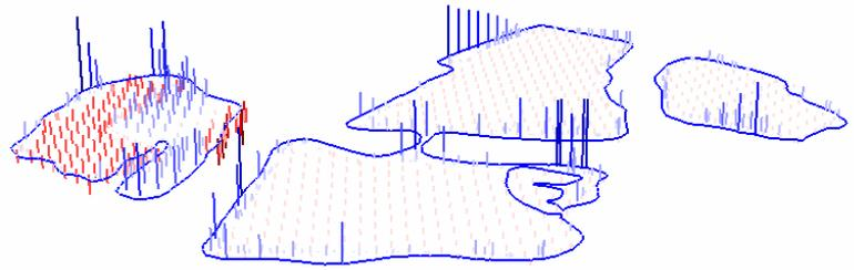
Figure 6: Height differences between the original heights of the DTM and the estimated heights of the optimization process (vertical exaggeration factor: 30), object: lake
