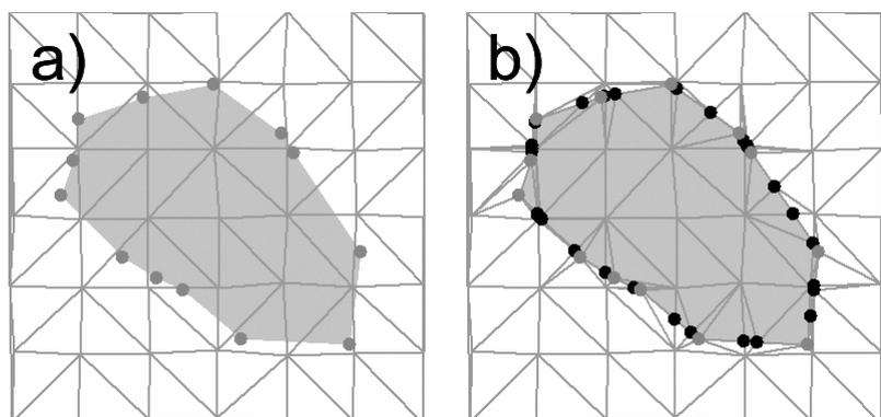
Figure 2: Integration of a DTM and a topographic object “lake“, a) original DTM TIN and object “lake“, b) integrated data set
