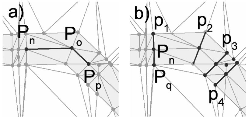
Figure 5: Equation and inequation constraints, a) maximum slope and maximum slope difference, b) horizontal profile and points belonging to a plane
