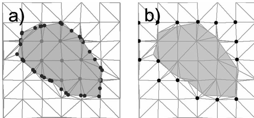
Figure 4: Equality and inequality constraints of a horizontal plane, topographic object “lake“, a) points inside the lake and points of the waterline, b) points of the neighbouring terrain
