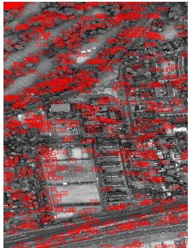
Figure 4: Distribution of the tie points on a display detail of one image (north is left).
