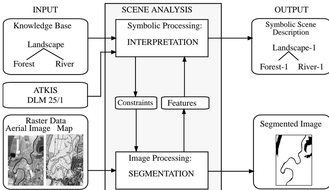
**Fig. 1:** Architecture of the knowledge based scene analysis system
