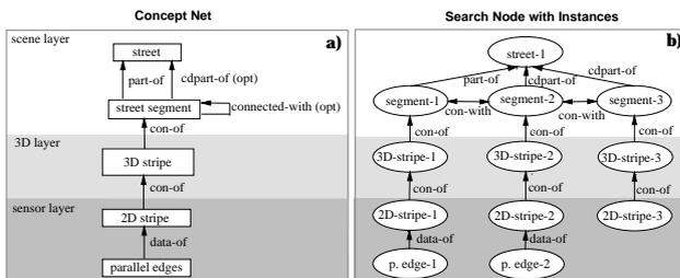
Figure 1: Semantic net for road detection (part)
