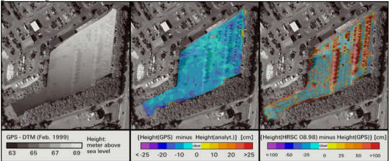
figure 2: DEM based on GPS-measurements 1999 (left), calculated differences between GPS-measurements and analytical measurements 1993 (middle), calculated differences HRSC-DEM and GPS-measurements
