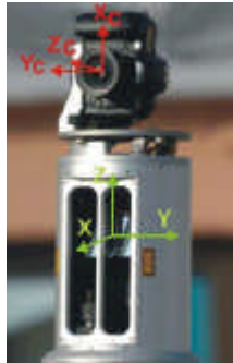
Figure 1: Combined sensor – laser scanner with mounted camera (RIEGL, 2004)
